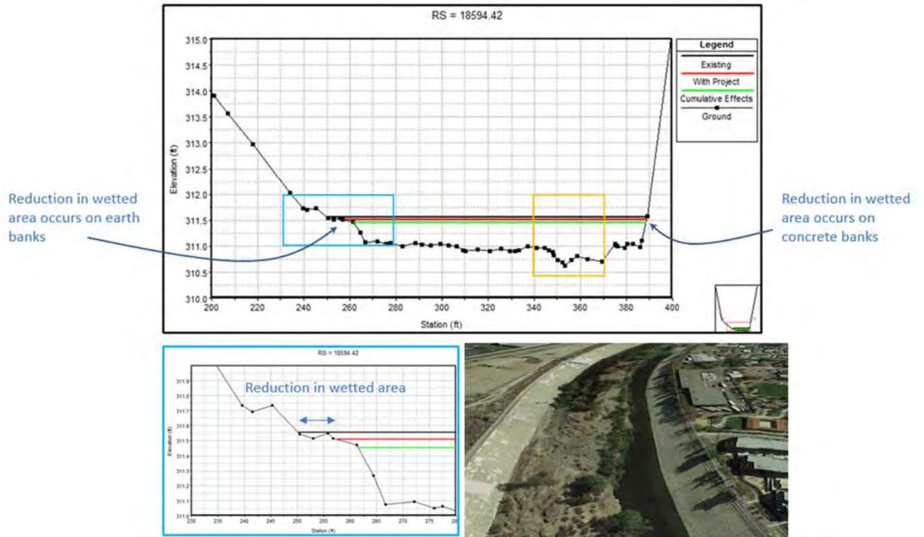
**Figure 10. Modeled water surface elevations for ARBOR reach 6 under existing, with-project and cumulative effects conditions, for August 2008 Condition**
