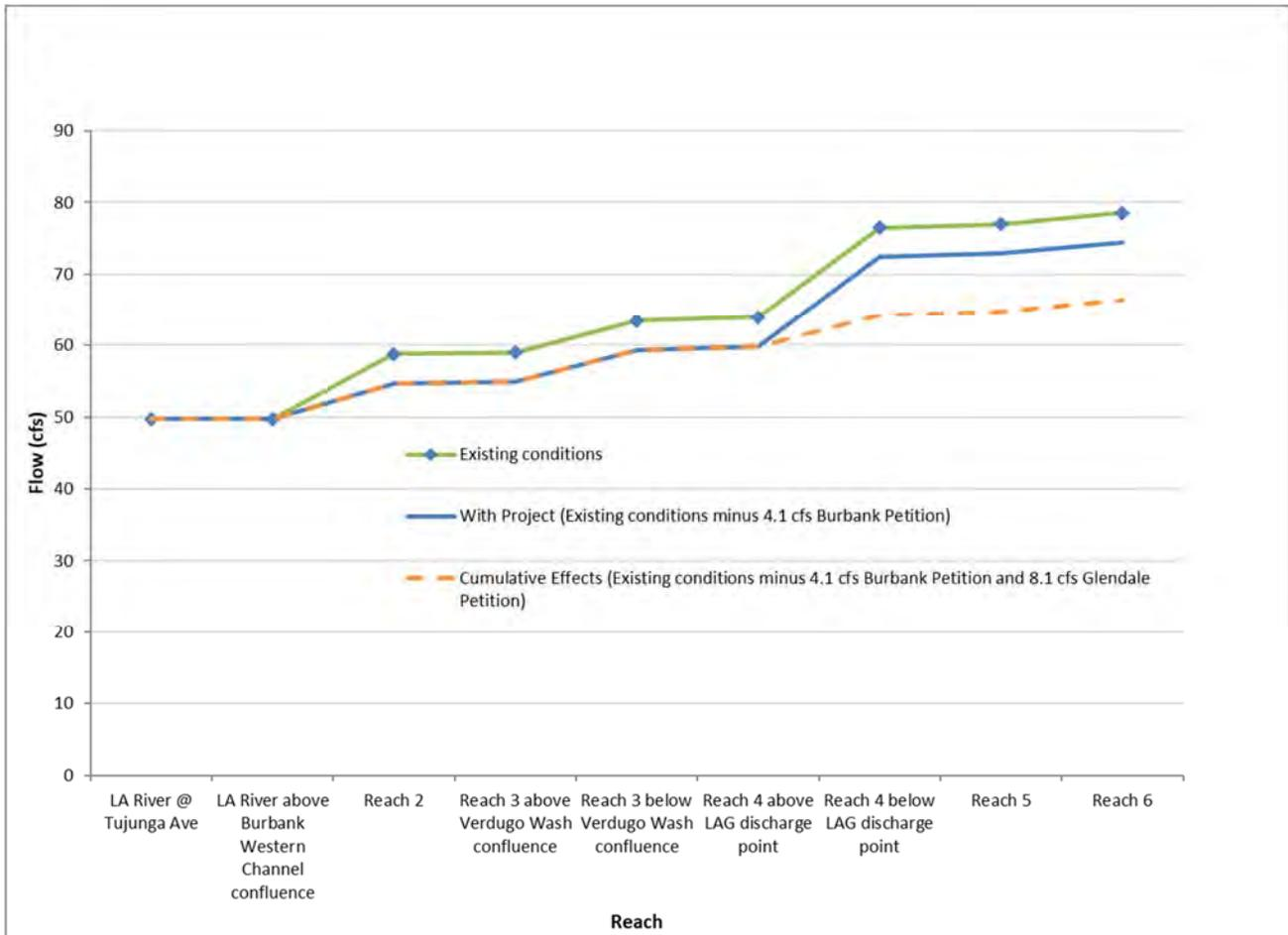
**Figure 4. Schematic of flow for each reach in the study area under existing, with-Project and cumulative effects scenarios**
