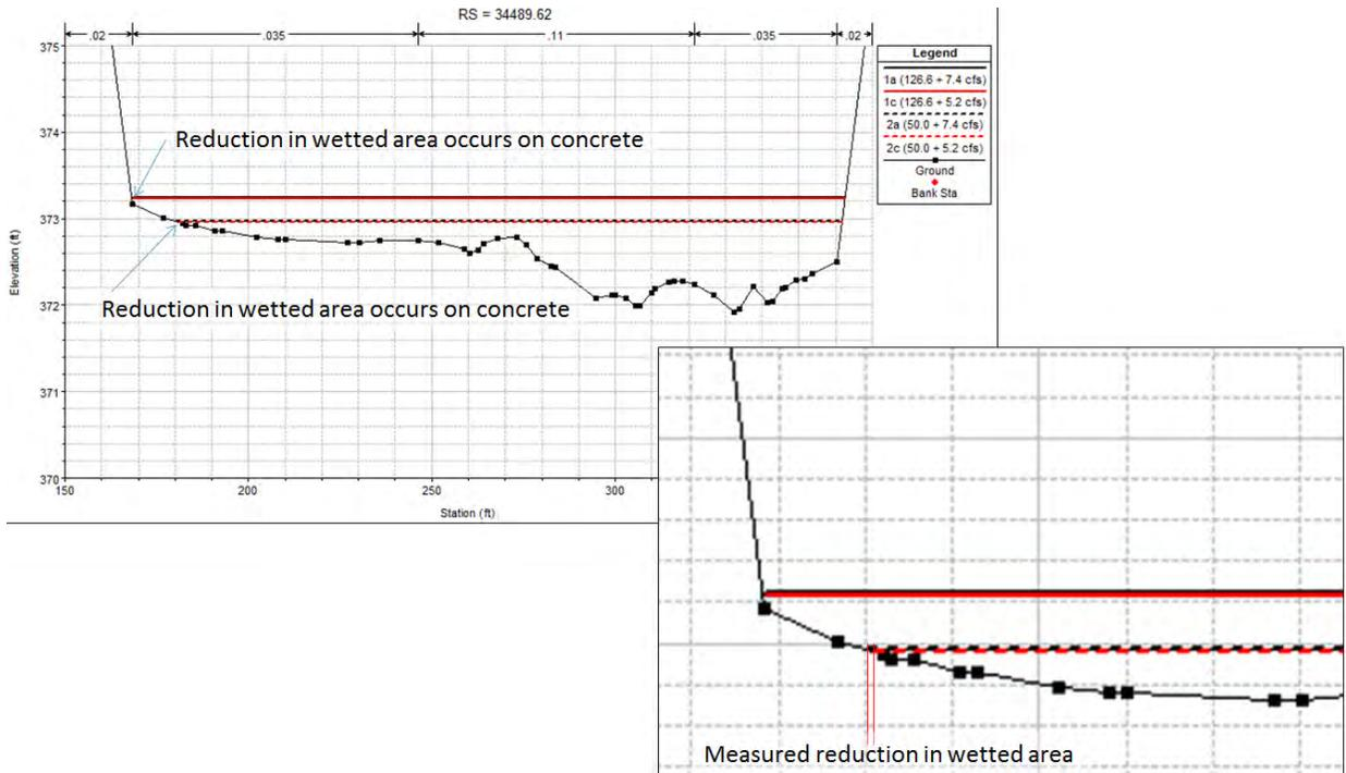
Figure 6 Example cross section used to estimate change in wetted area
