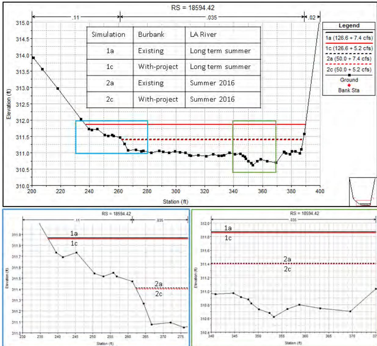
**Figure 5. Modeled water surface elevations for ARBOR reach 6 under existing and with-project conditions, for long-term summer and 2016 baseline condition Los Angeles River flows**
