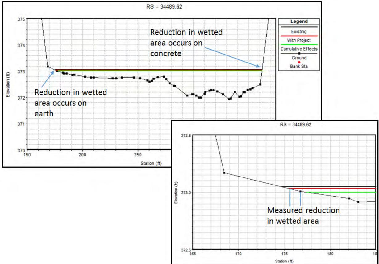
Figure 11. Example cross section used to estimate change in wetted area
