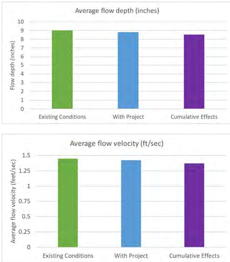
Figure 6. Average flow depth and velocity under Project and Cumulative effects
