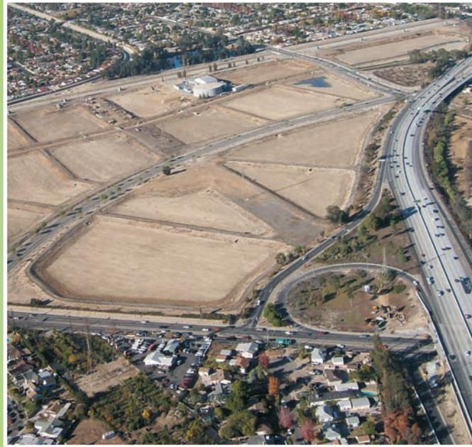
BWP plans to spread seasonally available water at the Pacoima spreading ground facility to increase ground water inventory for use during droughts or emergencies.
