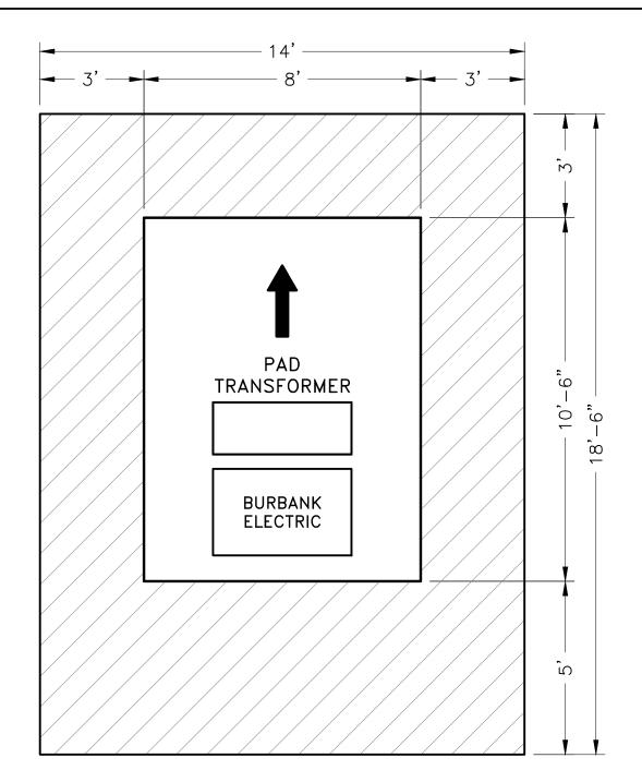
8' X 10'-6" THREE PHASE TRANSFORMER PAD CLEARANCE REQUIREMENTS
