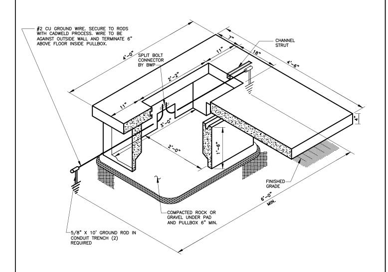
4'-6" X 4-0" TRANSFORMER PAD, WITH 3'-0" X 2'-0" X 1'-6" BOX JENSEN PRECAST ASSEMBLY MODEL NO. PD4854-T4-17B; HUBBEL QUAZITE NON-CONCRETE PAD MODEL NO. PH4481826F4S AND MODEL NUMBER PG2436BA18; OR EQUIVALENT FOR ALL SINGLE PHASE TRANSFORMER INSTALLATIONS (MAXIMUM TRANSFORMER WEIGHT-3000 POUNDS).
